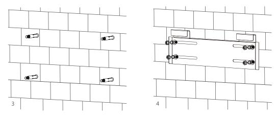
**Step 3.** Hang the inverter onto the wall-mounting bracket and lock the inverter on the wall using 2 self-tapping screws on the top of the inverter, lock the safety screws on the left and right sides.
