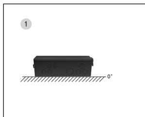
1. Place the inverter horizontally on a stable surface (such as a table or the floor) to ensure stability during operation and to prevent debris from falling inside.
