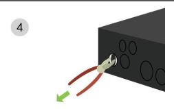
4. Use pliers to grip the loosened knockout cover and gently pull it out.
