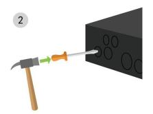
2. Select the appropriate knockout hole based on the cable routing, then lightly tap the edge of the knockout hole with a hammer and screwdriver.
