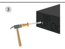
3. Loosen the knockout cover. Avoid using excessive force to prevent damaging the casing or internal circuits.
