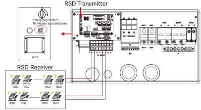
In case of emergency, press the rapid shutdown button that cut off the RSD power supply, thus stopping the inverter AC output, and the PV conductors voltage will be reduced to less than 30V within 30 seconds.
