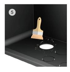
5. Use a brush or vacuum cleaner to clear any metal shavings that have fallen inside, ensuring no debris remains inside the device.
