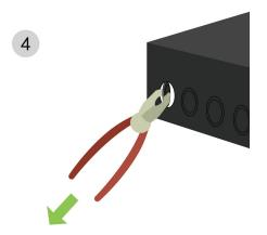
4. Use pliers to grip the loosened knockout cover and gently pull it out.
