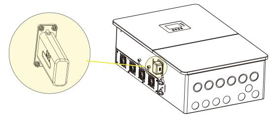
When installing the inverter, make sure that the dongle is connected to the inverter.
