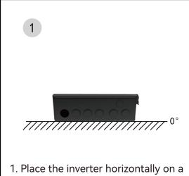
1. Place the inverter horizontally on a stable surface (such as a table or the floor) to ensure stability during operation and to prevent debris from falling inside.
