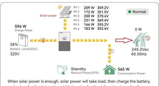
when solar power is enough, solar power will take load, then charge the battery, and at last feedback into the grid (when the feedback function is enabled).
