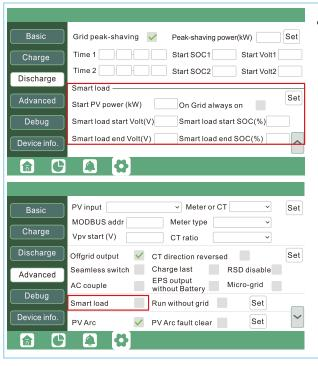
Smart Load: If you enable it, inverter will supply power to this load when the battery SOC and PV power is above a user setup value. e.g. Smart load start SOC=90%, Smart load end SOC=85%, Start PV power=300W, it means: When the PV power exceeds 300W, and the battery system SOC gets to 90%, the Smart Load Port will switch on automatically to supply the load which is connected on this side. When the battery reaches SOC<85% or PV power<300w, the Smart Load Port switch off automatically.
