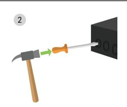
2. Select the appropriate knockout hole based on the cable routing, then lightly tap the edge of the knockout hole with a hammer and screwdriver.
