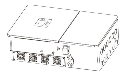
b. Remove the fan fixing.
