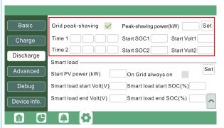
• Grid peak-shaving 8 Grid peak-shaving power(kW): Is used to set the maximum power that the inverter will draw from its grid power. And the Peak-shaving power needs to be set to more than 0.2(kW).
