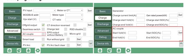
Users need to enable AC coupling function when they connect existing on grid system to smart load. Start SOC(%): The SOC at which the AC coupled inverters are turned on when in off-grid mode. 50%~70% recommended
