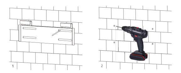
**Step 2.** Install and tighten the expansion bolts into the holes. Then use the corresponding nuts and washers (packaged together with the expansion bolts) to install and fix the wall-mounting bracket on the wall.
