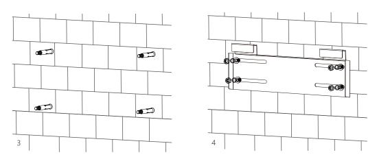
**Step 3.** Hang the inverter onto the wall-mounting bracket and lock the inverter on the wall using 2 self-tapping screws on the top of the inverter, lock the safety screws on the left and right sides.
