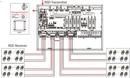
In case of emergency, press the rapid shutdown button that cut off the RSD power supply, thus stopping the inverter AC output, and the PV conductors voltage will be reduced to less than 30V within 30 seconds.
