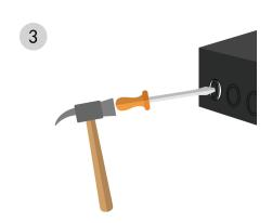
3. Loosen the knockout cover. Avoid using excessive force to prevent damaging the casing or internal circuits.
