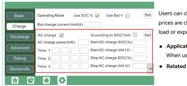
Users can charge batteries with grid power when electricity prices are cheap, and discharge battery power to supply load or export to the grid when electricity prices are high.
