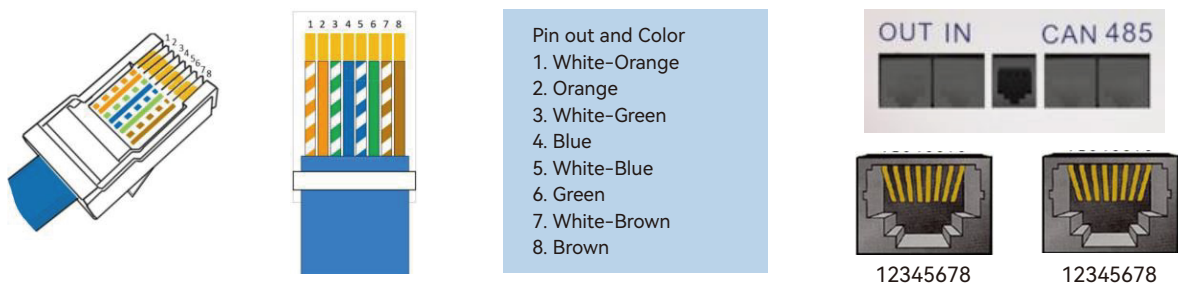
Figure 2-2 CAN, RS485, OUT, IN interface definition
