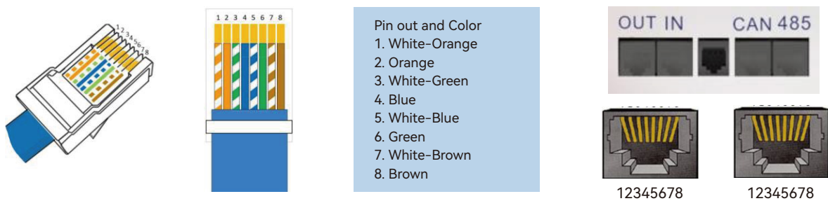
Figure 2-2 CAN, RS485, OUT, IN interface definition
