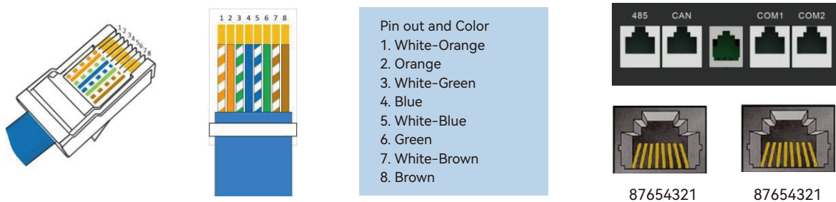
Figure 2-2 CAN, RS485, COM1, COM2 interface definition
