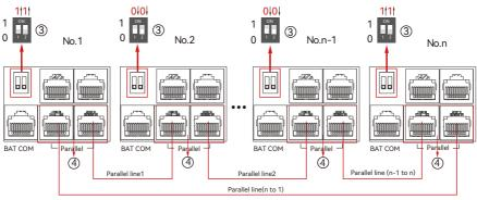
Step 2. Please put the CAN communication PIN to on status for the first and the end inverter
