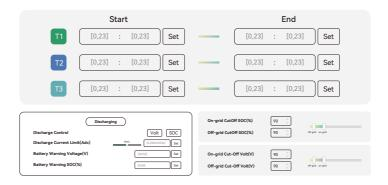
2. AC Charge function Disable: The system will not use AC to charge the battery (except Li-ion BMS set force charge flag)
