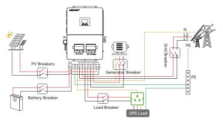
When properly wired and configured, the generator, if compatible with remote start, will start automatically when the battery voltage / SOC is lower than the cut-off value or there is a charge request from the BMS. When the generator is running, it will charge the batteries and excess AC power will be diverted to the AC output (LOAD) to power loads.
