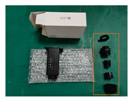
2. Disassemble the gland connector.
