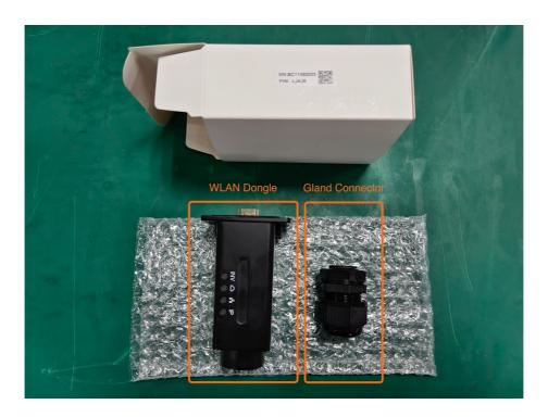
Open the box, check the two parts, WLAN dongle and gland connector.
