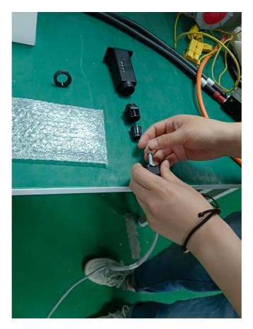
4. Get the ethernet cable through the gland connectors one by one.
