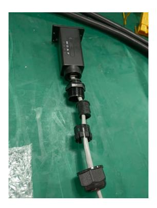
6. Plug the RJ45 head(crystal head) into WLAN dongle once all 4 gland connectors were installed through.
