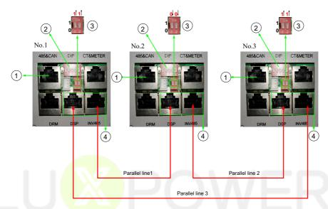
If there are more than three inverters parallel in this three-phase system, only two of the longest distance need to be dialed toward "on" position: 1 1 1 , and others keep off: 0 0
