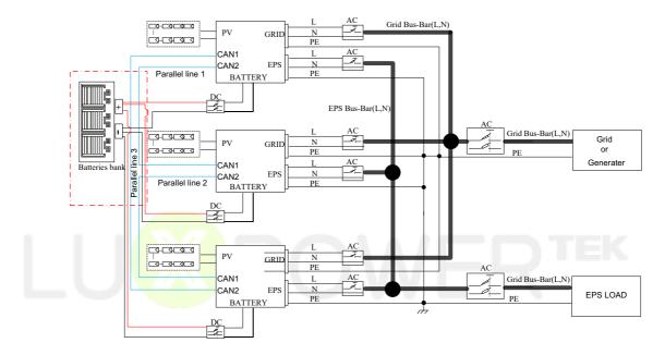
■ If you connect one battery bank shared by multiple inverters as the diagram above, please enable "Battery shared".
