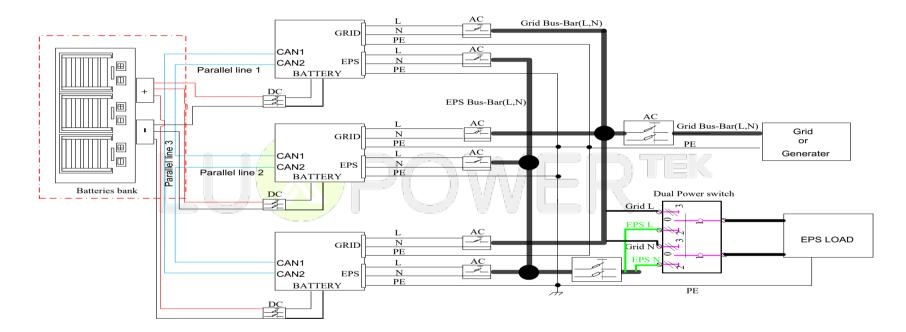
■ If you connect one battery bank shared by multiple inverters as the diagram above, please enable "Battery shared".
